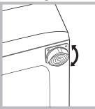
Your machine may make a considerable amount of noise if the two front feet have not been adjusted correctly.
